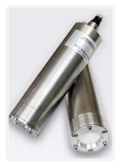
No internal moving parts or pumps, hence lower failure risk and lower power drain. Inherent to the technology, and also dependent on detector manufacturing and tuning, all parameters such as sensitivity, power consumption, response time and response behavior are linked together. Following specifications are indicative, we can select and tune the detectors to meet your requirements.
